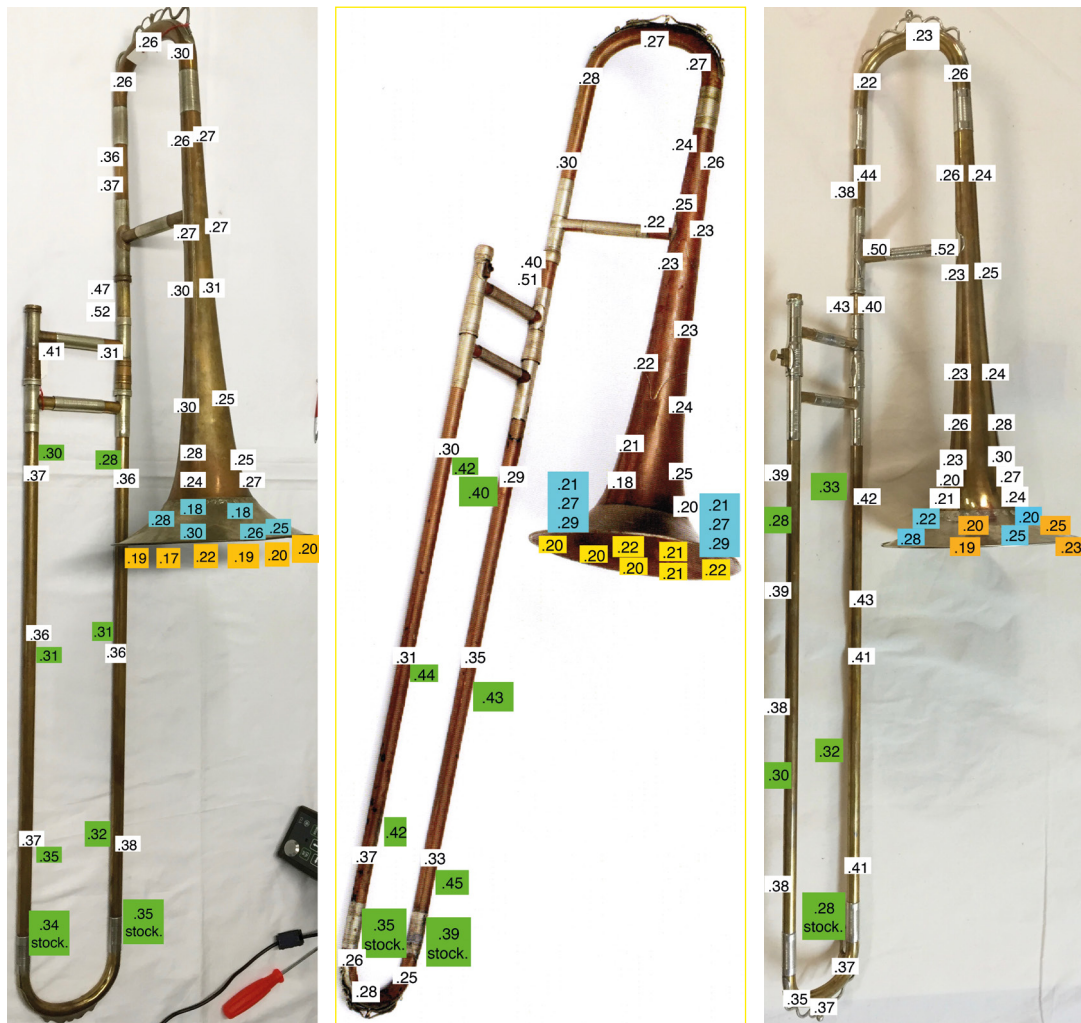
Figs. 21–23 Three typical trombones by J. C. Penzel (left, private collection Sebastian Krause), F. A. Heckel (middle, private collection Jürgen Kamjunke) and Ed. Kruspe (right, private collection Rainer Egger); in green: inner slide measurements (stock. = stockings), in blue: garland, in orange: bell below the garland.
