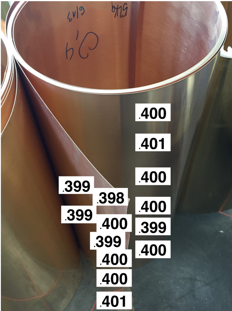
Fig. 16 A modern roll of brass at Egger's workshop. The 14 measurements show that the 0.4 mm thickness is within a tolerance of 1/1000 mm.
