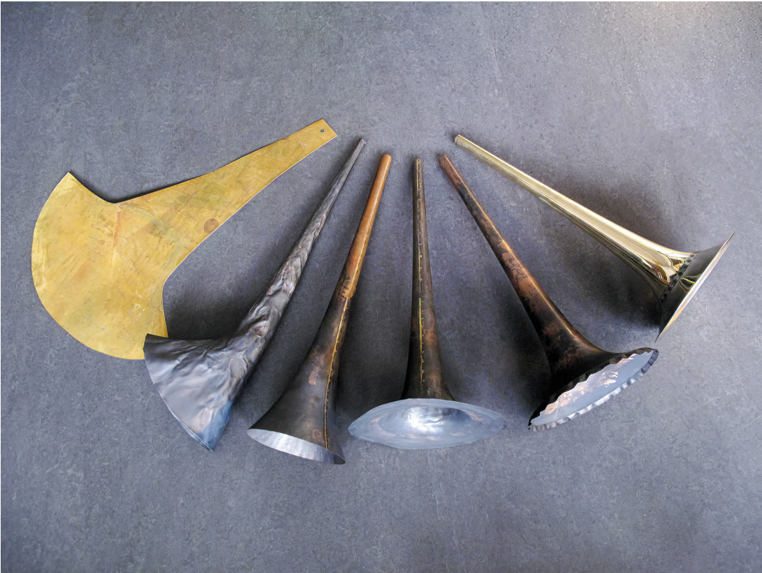
Fig. 1 The steps of bell-making from left to right: the sheet metal, after soldering, the symmetrical shape, the opened bell, after shaping on the mandrel, and the finished Egger Romantic tenor trombone bell (Foto: AS).
