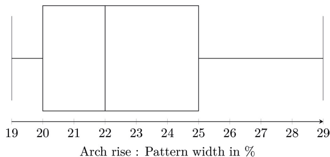
Fig. 5 Ratio of arch rise to pattern width.
